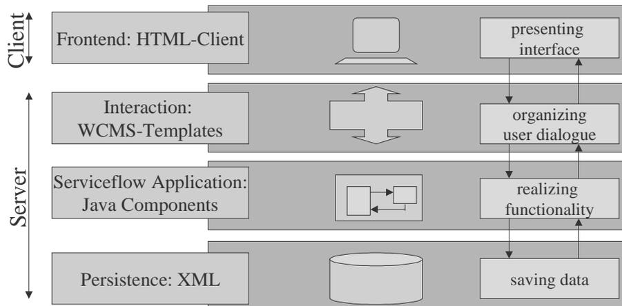
Figure 4. IT architecture for a web-based service point
